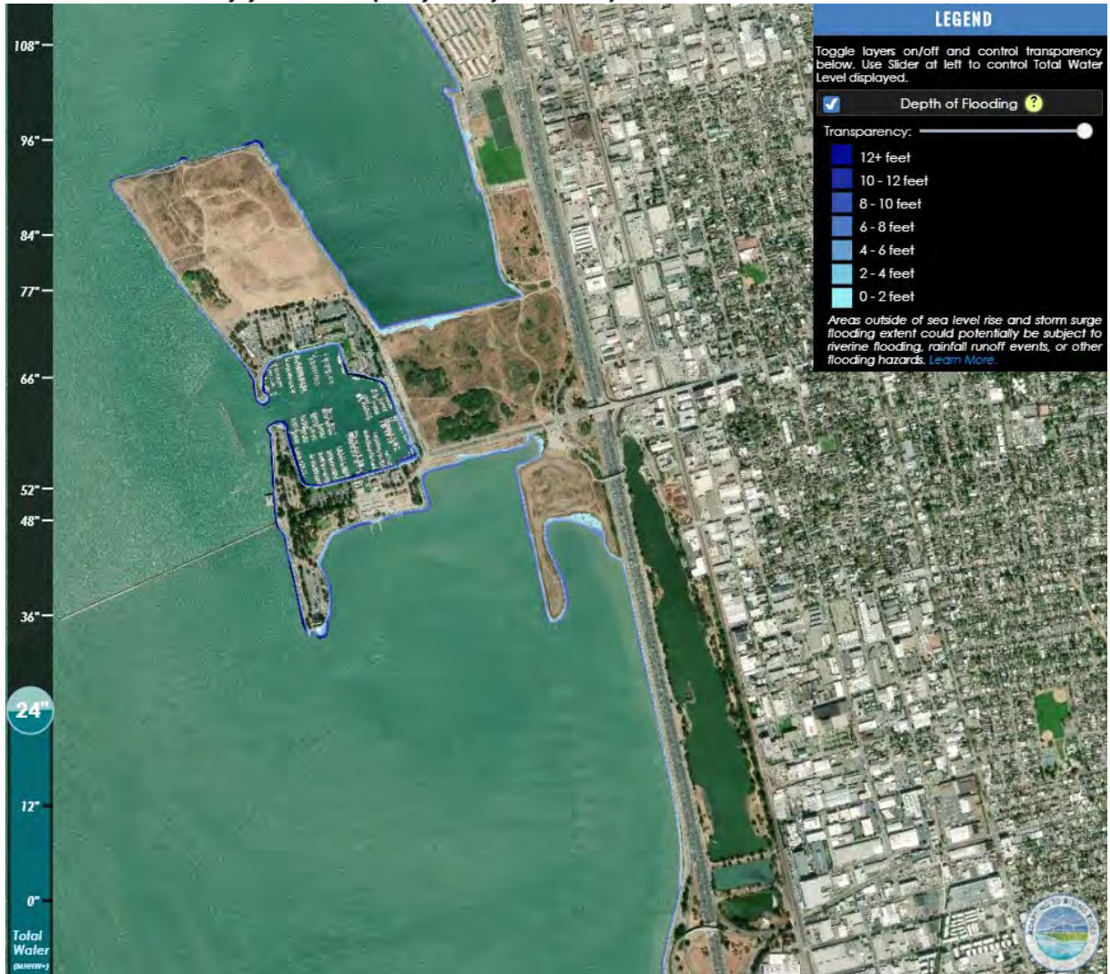
Map 30. Berkeley Shoreline Areas Prone to Permanent Inundation due to 2-ft of Sea Level Rise by year 2100 (Very likely scenario)
